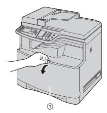
2 Unlock the drum cartridge cover by pushing the tabs (2) in the direction of the arrows.
